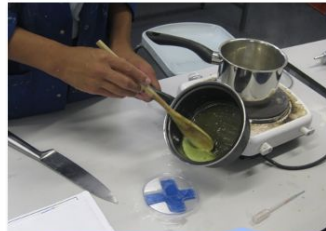
Pouring molten glycerine into vacuum formed molds
