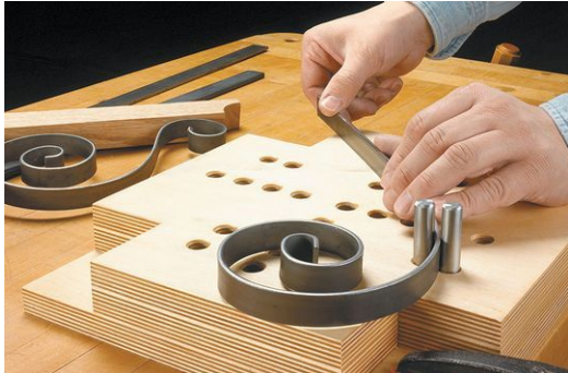
Bending with a jig
